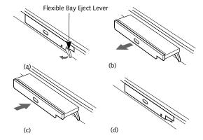
Figure 2-17 Removing/Installing a device in the Flexible Bay
